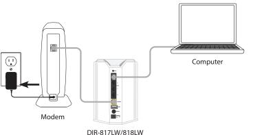
Plug the power adapter into your router and connect to an available power outlet or surge protector. If the Power LED does not light up, press the Power button on the back of the router.
