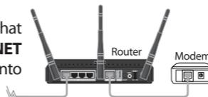
**Step 5** - Reconnect the power adapter to your cable or DSL broadband modem and wait for two minutes.
