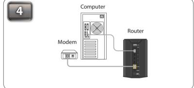
Position your router close to your modem and a computer. Unplug the Ethernet cable from your modem (or Plug one end of the included blue Ethernet cable that came with your router into the yellow port labeled **INTERNET** on the back of the router. Plug the other end of this cable into the Ethernet port on your modem.
