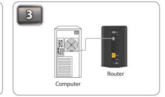
existing router if upgrading) that is connected to your computer. Plug it into the black port labeled 1 on the back of your router. The router is now connected to your computer.
