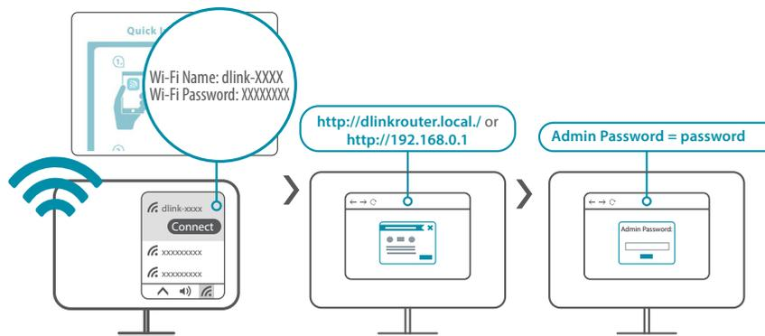
**TECH TIP:** Consider using the same Wi-Fi name and password as your old router. This will allow your existing Wi-Fi devices to automatically connect to your new router.
