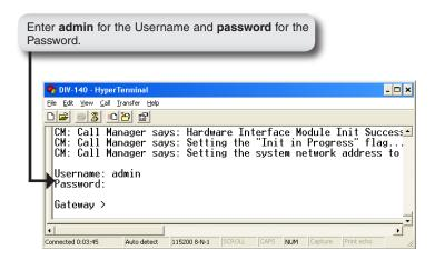
It may be necessary to change the IP address of the DIV-140 to match your local network. To change the IP address of the DIV-140, use the following commands and procedure below:
