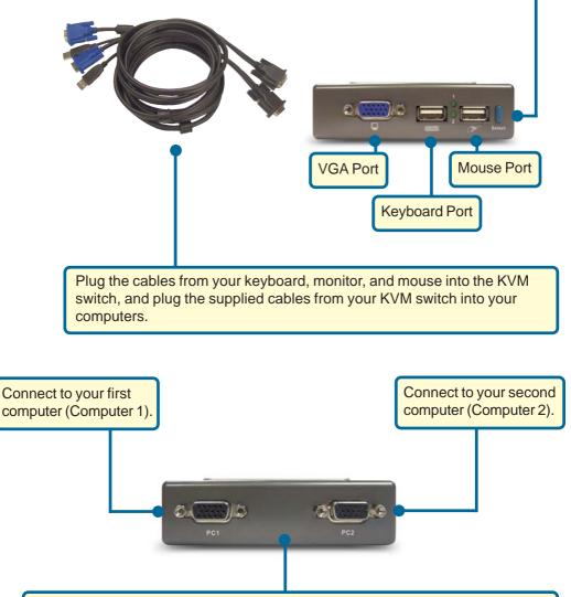
The DKVM-2U is assembled with the supplied KVM cables fastened to the PC1 and PC2 ports. Plug the cable from PC1 into your first computer (Computer 1), and plug the cable from PC2 into your second computer (Computer 2).
