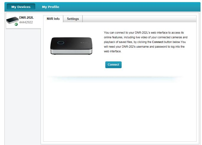
To connect to your NVR click on the **Connect** button and provide your password to complete the login process. After you have connected to the NVR, you will be taken to the Live Video page. (Refer to "**Live Video**" on page 21)
