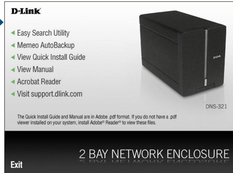
The Easy Search Utility will load and detect any DNS-321 devices that are on the local network. If the DNS-321 you are working with does not show up in the device list, click **Refresh**.
