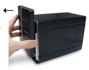
Insert a 3.5" SATA hard drive into an available drive bay. Make sure to align the drive connector to the endpoint in the DNS-321. Gently push the drive in until it connects.
