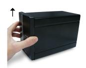
Once the faceplate is unlatched, pull it off of the device, exposing the drive bays.
