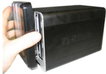
3. Insert a 3.5" SATA hard drive into each available drive bay. Make sure to align the drive connectors to the endpoints in the DNS-323. Gently push the drive in until it connects.
