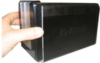
2. Once the faceplate is unlatched, pull it off of the device, exposing the drive bays.
