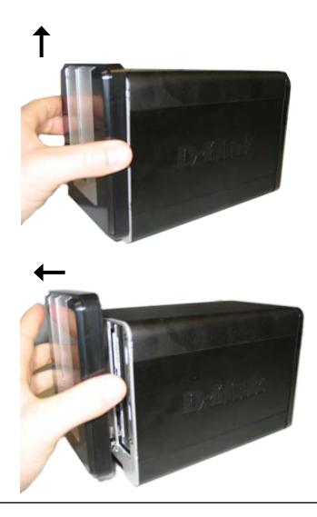
3. Insert a 3.5" SATA hard drive into each available drive bay. Make sure to align the drive connectors to the SATA connectors on the bottom edge inside the drive bay of the DNS-323. Gently push the drive in until it connects. When a drive is inserted properly, you will feel it "seat" into the connector. Some hard drives that are thin or oddly shaped may need to be guided carefully into position. If a drive is not properly seated, the light will not illuminate after powering on the device.
