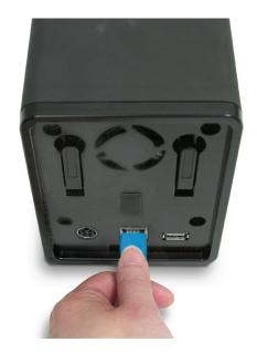
6. Connect the power adapter to the power receptacle.
