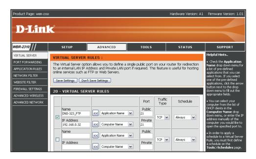
If you use an FTP port other than 21, then users accessing the FTP server using an FTP client will have to specify the non-standard port, and users who are using a browser will have to specify the port in the URL (e.g. ftp://ftp.dns323.com:3000, where the FTP port is 3000).
