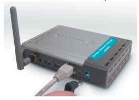
Attach your USB drive(s) to the USB port(s) on the rear panel of the DNS-G120. The USB LED on the front panel will blink until the drive has been installed. Once the USB LED is solid green, your USB drive is ready for use.
