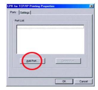
Type in the IP address of the DP-101P+. Make sure the **Port Name** is accurate. The **Port Name** at right is just an example. (*Please refer to page 13 in this manual to find the Port Name in the Server Device window.)
