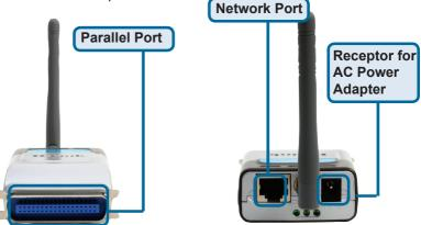
Then, plug one end of the power adapter into the DP-G301 and the other end into your electric outlet. The DP-G301 will turn on and begin a self-test.
