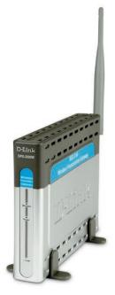
The DPG-2000W uses 802.11g technology for fast and responsive display of images, presentations and applications via projector or on a monitor.
