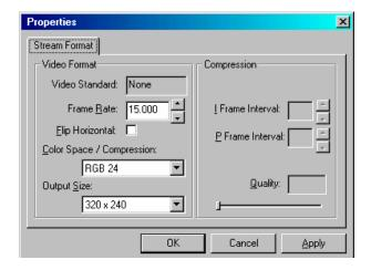
In the **Frame Rate** display you have the options from 7.5 frames per second (fps) up to 30 fps.
