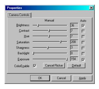
Under the **Camera Controls** tab, make the appropriate adjustments from the menu list to fine tune the image related parameters such as Brightness, Contrast, Saturation, Sharpness, Hue, Backlight, and Exposure or set to Default
