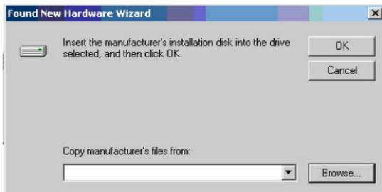
The driver is located in the folder named **Bcm63xx\_WHQL\_usb\_driver**. The file name is **usbdsur.inf**. Click **Open** to proceed with the installation.
