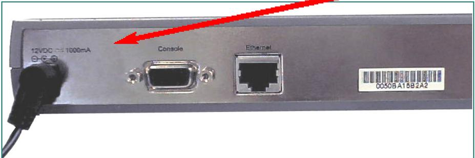
Once the unit power is on, insert one end of the included **Ethernet cable** into the DSL-300's Ethernet port, and the other end into the Ethernet port on the NIC installed in your PC.
