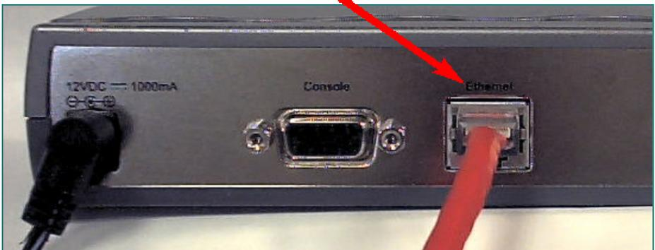
*If the cable connection is good, a green LED on the front of the DSL-300 labeled Ethernet/Link will glow steadily.*
