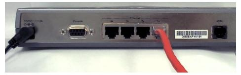
If the cable connection is good, a green LED on the front of the DSL-504 labeled Ethernet/Link will glow steadily.
