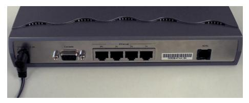
Once the unit power is on, connect one end of the included Ethernet cable to the DSL-504's ethernet port and connect the other end of the cable into the NIC which is installed in your computer.
