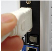
High-Definition Multimedia Interface (HDMI) supports standard, enhanced, or high-definition video, plus multi-channel digital audio on a single cable.
