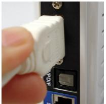
High-Definition Multimedia Interface (HDMI) supports standard, enhanced, or high-definition video, plus multi-channel digital audio on a single cable.
