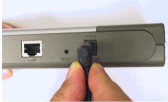
Connect an Ethernet cable to the Ethernet jack located on the back of the DSM-602H/604H.
