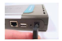
Connect an Ethernet cable to the Ethernet jack located on the back of the DSM-622H/624H.
