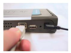
After the Ethernet cable is securely connected, connect the other end of the Ethernet cable to your network router or switch. (The router is pictured here.)
