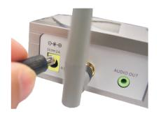
Connect your speaker's audio cable to the **Audio Out** connector located on the rear panel of the DSM-100BT. For connection to a speaker system with RCA outputs, you can use the included RCA to 3.5mm audio converter connector for installing the DSM-100BT.
