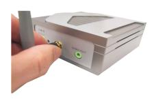
Connect one end of the power adapter to the power connector located on the rear panel of the DSM-100BT and the other end to an available power strip or wall outlet. The Power LED indicator will light green to indicate that the DSM-100BT is powered on.
