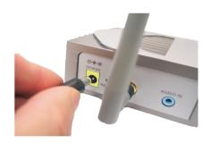
Connect your audio player's audio cable to the **Audio In** connector located on the rear panel of the DSM-110BT using the included 3.5mm cable. For connection to a stereo sytem with RCA outputs, you can use the included RCA to 3.5mm audio converter connector for installing the DSM-110BT.
