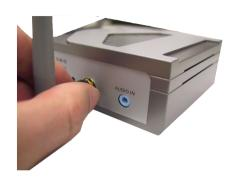
Connect one end of the power adapter to the power connector located on the rear panel of the DSM-110BT and the other end to an available power strip or wall outlet. The Power LED indicator will light green to indicate that the DSM-110BT is powered on.
