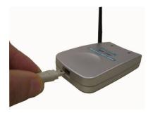
Connect the flatter, larger end of the included mini USB cable to an available Type A USB slot on the rear panel of your computer. The Power LED indicator will light green to indicate that the DSM-120BT is powered on.
