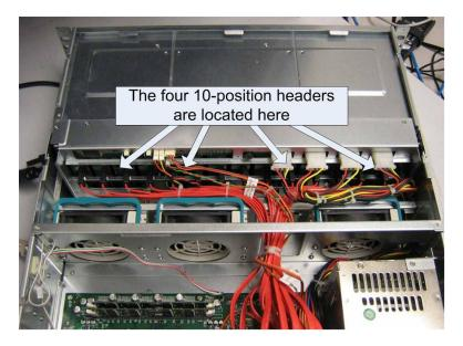
Figure 4: Identifying the four 10-position headers
