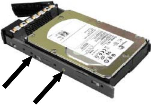
To install SATA drives with Bridge Board (DSN-654), fit the Bridge Board first
