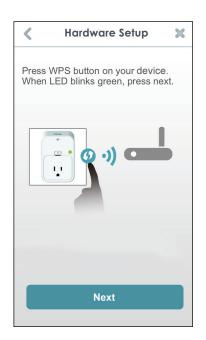
After about two minutes, the Status LED will turn solid green. This indicates that the Smart Plug has successfully connected to your wireless router. Tap **Next** to continue.
