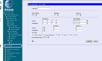
**Protocol-**Select **IGMP**, **TCP**, **UDP** or **All** to pass or block packets of that protocol type.
