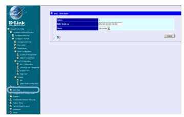
**State -** This toggles Disable and Enable for the MAC address filtering function for this index
