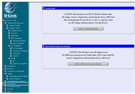
Before performing a Factory Reset, be absolutely certain that this is what you want to do. Once the reset is done, all of the device's settings stored in NV-RAM will be erased and restored to values present when the device was purchased.
