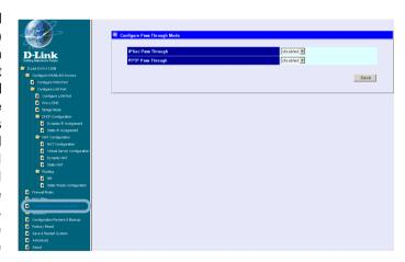
**PPTP Pass Through / IPSec Pass Through -** This toggles Disable and Enable for the Pass Through function.
