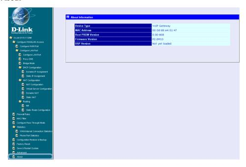
This read-only window displays information about the DVG-1120M VoIP Station Gateway such as: Device Type, MAC Address, Boot PROM Firmware, Firmware Version, and DSP Version. The DSP Version will list "Not yet loaded" until you initialize your unit.
