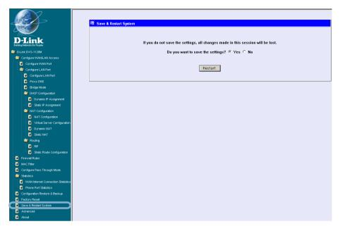
After the settings have been saved to NV-RAM, they will become the default settings for the device, and they will be used every time it is powered on, reset or rebooted. The only exception to this is a factory reset, which will clear all settings and restore the unit's settings back to their initial values, which were present when the device was purchased.
