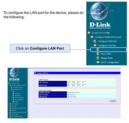
In this configuration menu, users can configure the LAN IP Address. (Recommended for advanced users.)
