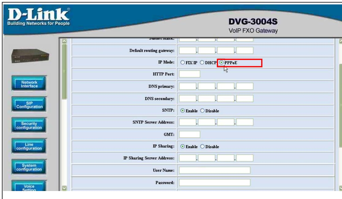
Figure 2.11: Switch to PPPoE function
