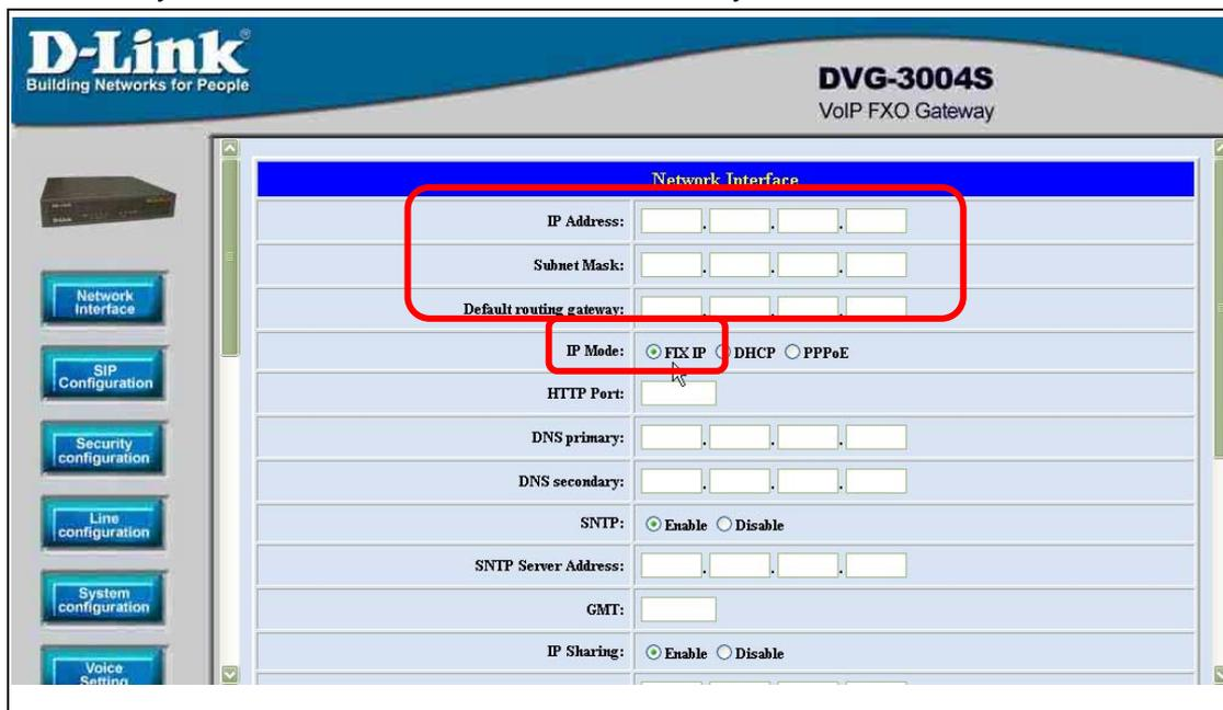
Figure 2.7: Configure the static ip address
