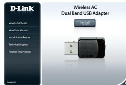
**Note:** If the CD Autorun function does not automatically start on your computer, go to **Start > Run**. In the run box type "D:\autorun.exe" (where D: represents the drive letter of your CD-ROM drive) and click **OK**.
