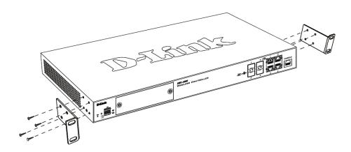
2. Use the screws provided with the equipment rack to mount the wireless controller into the rack.
