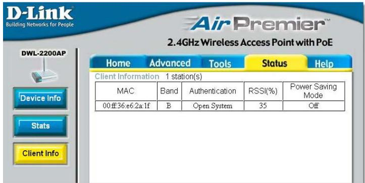
The screenshot shows the configuration interface for a D-Link Air Premier 2.4GHz Wireless Access Point with PoE. The 'Status' tab is selected, and the 'Client Info' sub-tab is active. A table displays information for one connected station.
