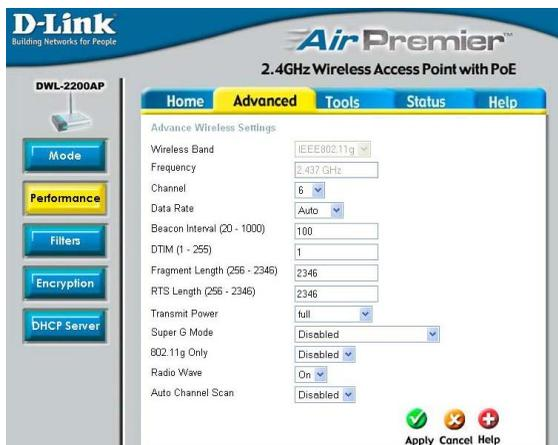
**Beacon Interval-** Beacons are packets sent by an access point to synchronize a network. Specify a beacon interval value. The default (100) is recommended.
