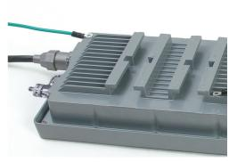
Step 2: Install the two dipole antennas to the antenna connector and attach the grounding wires.
