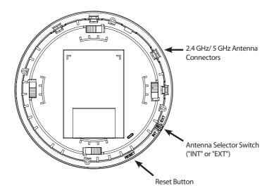
**Note:** The DWL-6600AP has an internal antenna. If you would like to use external antennas, please slide the selector switch to the "EXT" position and attach the antennas.
