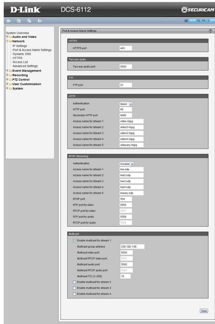
**Authentication:** Depending on your network security requirements, the Network Camera provides three types of security settings for streaming via HTTP protocol: disable, basic, and digest. If basic authentication is selected, the password is sent in plain text format, but there can be potential risks of it being intercepted. If digest authentication is selected, user credentials are encrypted using MD5 algorithm, thus providing better protection against unauthorized access.
