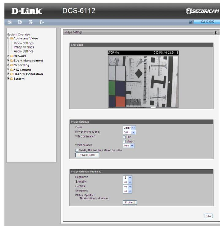
**Contrast:** Adjust the image contrast level, which ranges from -5 to +5
