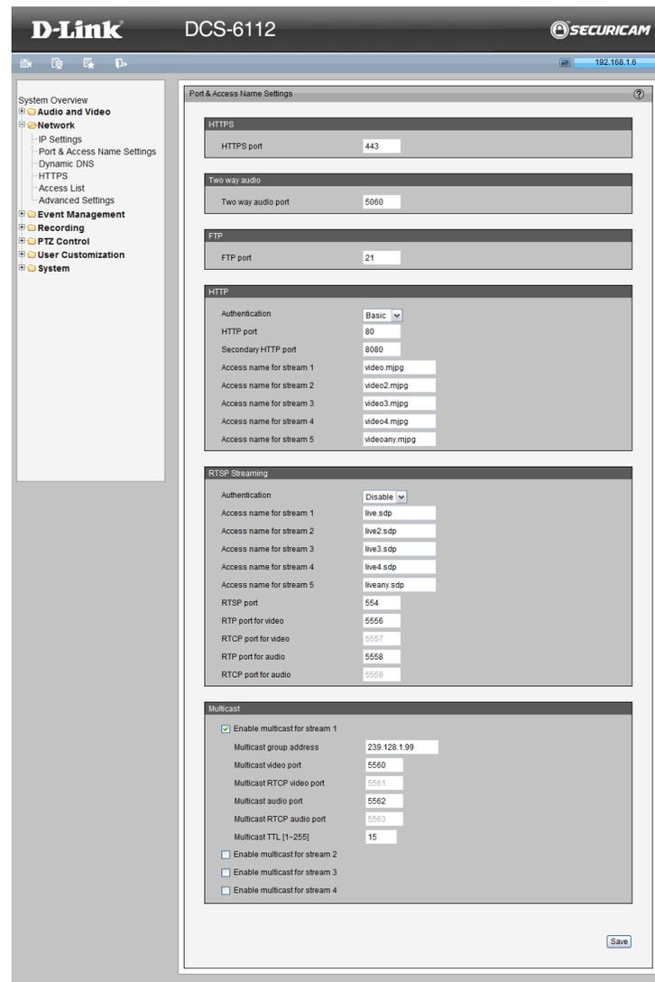
**Access name for stream 1 ~ 5:** This Network Camera supports multiple streams simultaneously. The access name is used to differentiate the streaming source. If you want to use an RTSP player to access the Network Camera, you have to set the video mode to H.264 / MPEG-4 and use the following RTSP URL command to request transmission of the streaming data.
