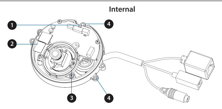
You can access the inside of the DCS-6210 by loosening the three security screws, then lifting the cover off of the camera.
