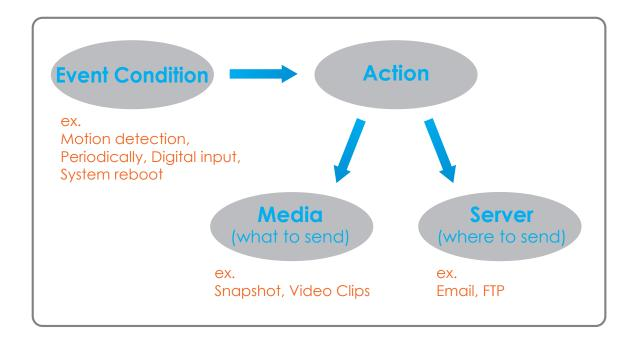
To start plotting an event, it is suggested to configure *Server* and *Media* columns first so that the Network Camera will know what action shall be performed when a trigger is activated.
