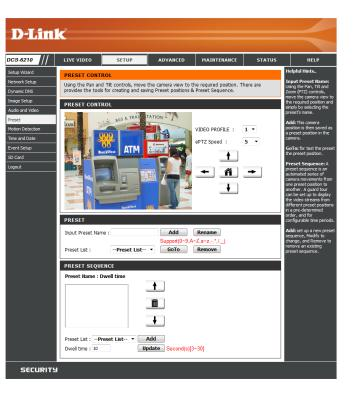
Preset List: To add a preset to the sequence, select it from the dropdown box at the bottom of this window, set the Dwell time to determine how long the camera view will stay at that preset, then click the Add button. The preset name will appear in the list followed by the dwell time for that preset view.
