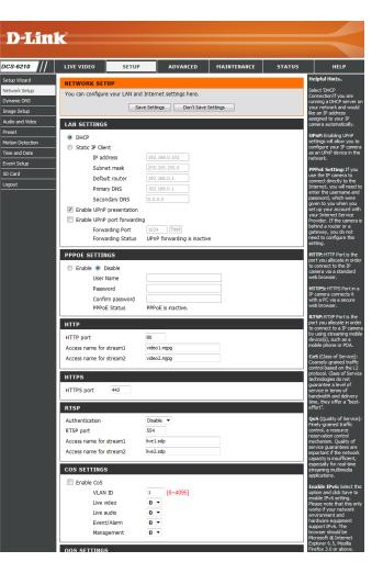
Enable UPnP Port Forwarding: Enabling this setting allows the camera to add port forwarding entries into the router automatically on a UPnP capable network.
