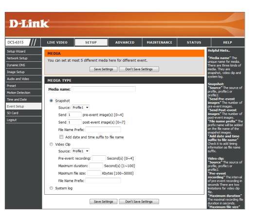
Add date and time Check this box to Add date and time as file name suffix to file name: suffix. Refer to the previous page for an example of how the file name will be displayed when this option is enabled.
