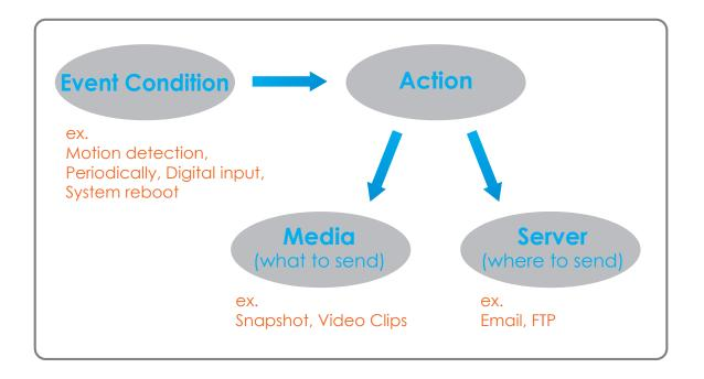
Instructions for setting an Event begin on the next page. Proper setup enables your DCS-6315 to perform as expected when a trigger is activated.
