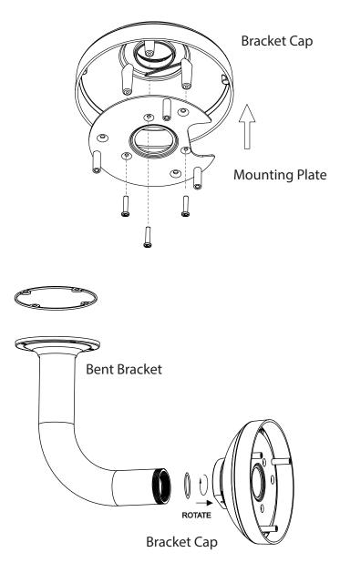
Section 2: Assembly and Installation
