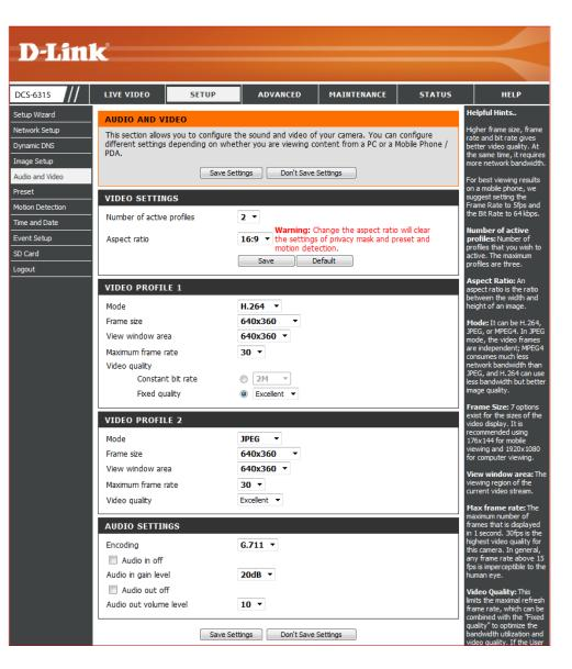
Maximum Select a number that represents video frames per frame rate: second. A higher frame rate means motion appears to be smoother, and requires more bandwidth. A lower frame rate will generally result in a stuttering motion, and requires less bandwidth.
