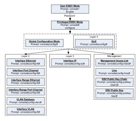
When starting a session, the initial mode is the User EXEC mode. Only a limited subset of commands is available in User EXEC mode. This level is reserved for tasks that do not change the configuration. To enter the next level, the Privileged EXEC mode, a password is required.
