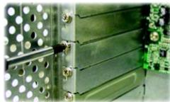
Locate an available PCI slot and insert the DFB-A5 carefully into the PCI slot.
