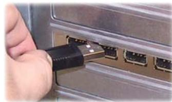
**Your computer will automatically detect and install the DFB-H7. Your installation is now complete! You may now connect USB 2.0 or USB 1.1 devices and/or Firewire devices to an available USB port or Firewire port on the front of the DFB-H7.**
