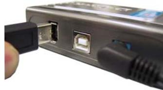
Plug the other end of the Firewire cable to an available Firewire port on your computer case.
