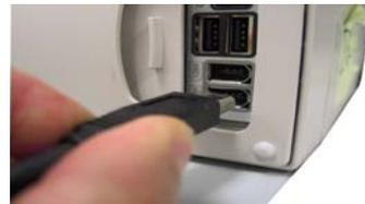
Plug the USB Type B connector (the smaller end of the cable) into the USB port located on the back panel of the DFB-H7.
