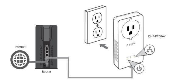
2. Plug in the other DHP-P700AV adapter in the room that you want to extend your network. The Power LED will turn on.
