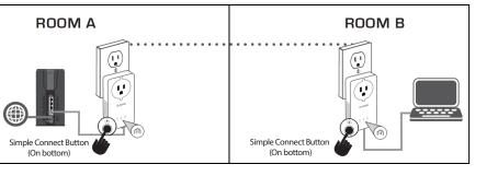
You can now connect another device using an Ethernet cable to the DHP-P700AV adapter. Verify that the Ethernet LED is lit. Your installation is completed.
