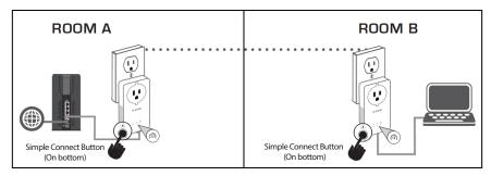
5 You can now connect another device using an Ethernet cable to the DHP-P700AV adapter. Verify that the Ethernet LED is lit. Your installation is completed.
