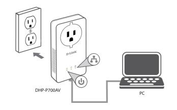
3 Verify that the PowerLine LEDs on both adapters are lit. If they are, the adapters are connected. If not, try another outlet.
