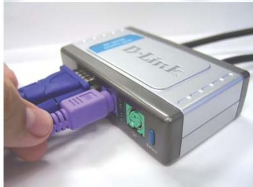
Attach your computer's 6-pin PS/2 male mouse connector to the DKVM-2K mouse port.
