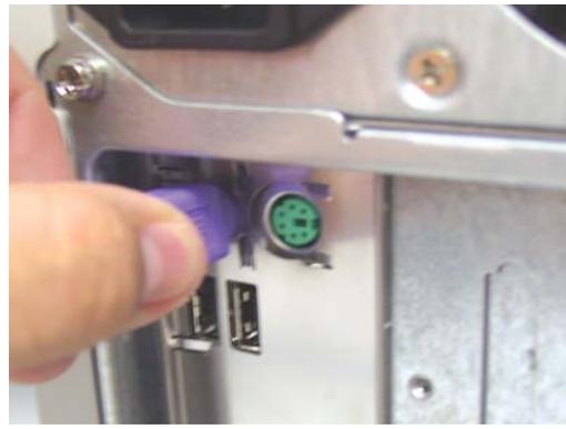
Attach the DKVM-2K's built-in mouse cable to the PS/2 mouse port located on the back of your computer case.
