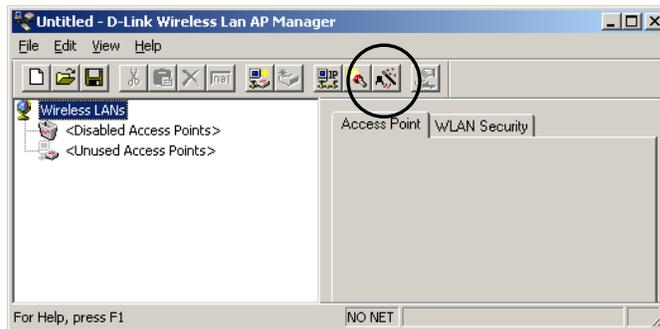
Once the IP address of Access Point software has been assigned go to **Start > Programs > D-Link Wireless LAN > Upgrade**
