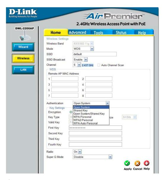
In WDS mode, the DWL-2200AP wirelessly connects multiple networks, without functioning as a wireless AP.
