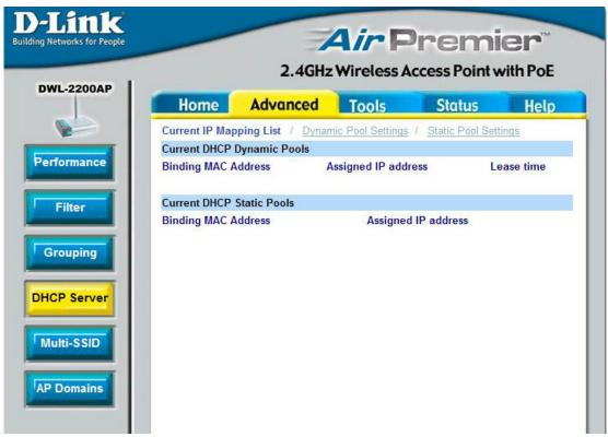
This screen displays information about the current DHCP dynamic and static IP address pools. This information is available when you enable the DHCP function of the DWL-2200AP and assign dynamic and static IP address pools.
